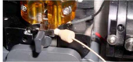
Closed loop nozzle installed
